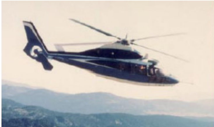
Figure 4.2 SA 365N – 1979 – C_x S = 1,05 \text{ m}^2
