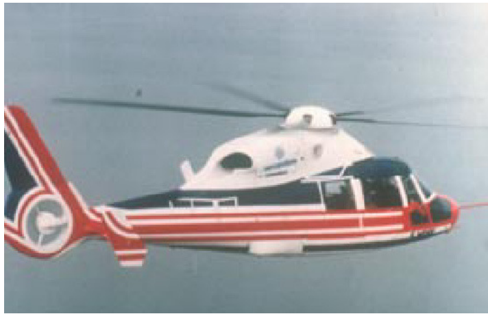
Figure 4.3 DGV 200 – 1989 – C_x S = 0,85 \text{ m}^2
